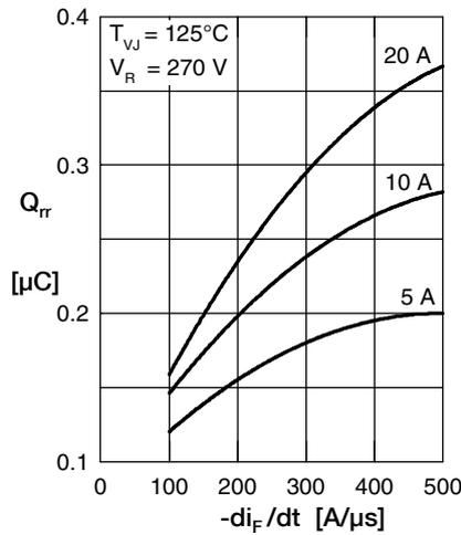
Fig. 2 Typ. reverse recov. charge  $Q_{rr}$  versus  $-di_F/dt$
