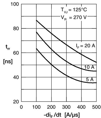
Fig. 5 Typ. reverse recov. time  $t_{rr}$  versus  $-di_F/dt$
