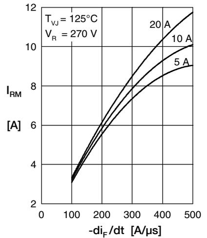
Fig. 3 Typ. reverse recov. current  $I_{RM}$  versus  $-di_F/dt$
