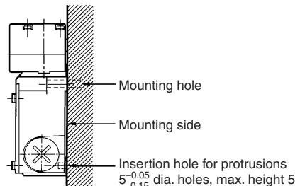
The D4BS can be mounted more securely by adding two protruding portions, each of which is 5 mm maximum in height and  $5^{-0.05}_{-0.15}$  mm in diameter as shown below.
