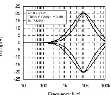
Fig.12 Treble Q vs Freq
