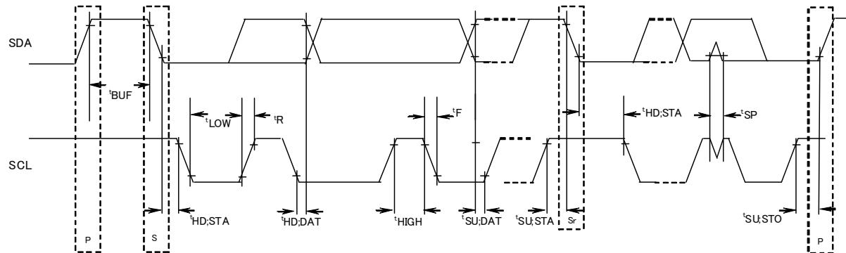
Fig.26 Definition of timing on the I<sup>2</sup>C-bus
