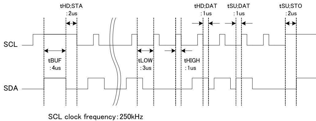
Fig. 27 A command timing example in the I<sup>2</sup>C data transmission
