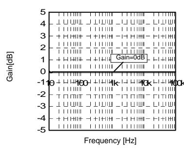
Fig.3 Gain vs Freq
