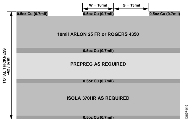
Figure 94. Evaluation Board Cross Sectional View
