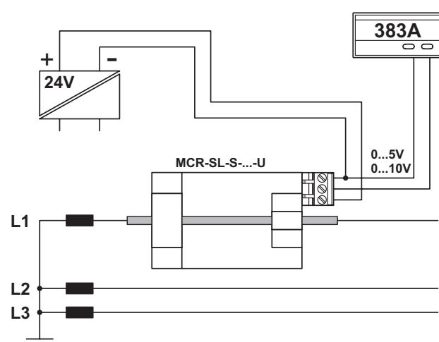
Figure 1 Current measurement
