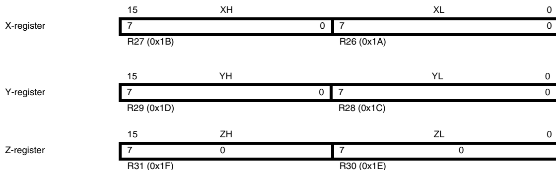
Figure 5-5. The X-, Y-, and Z-registers
