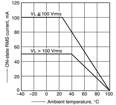
1-(4). ON-state RMS current vs. ambient temperature characteristics
