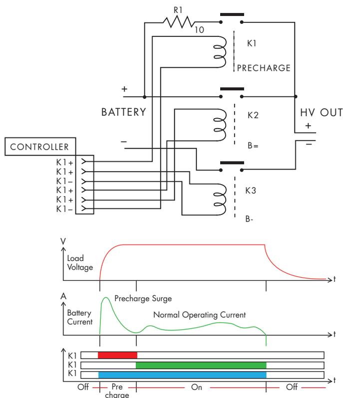
In its most basic form, the Precharge circuit operates as follows:
