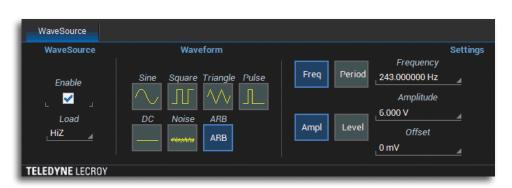
can be uploaded into the WaveSource to generate arbitrary waveforms. Familiar function generator controls are seamlessly integrated in to the WaveSurfer 3000 user interface simplifying the process of generating waveform stimulus and measuring the response with the oscilloscope. A rear panel BNC connector provides easy access to the generator output.
