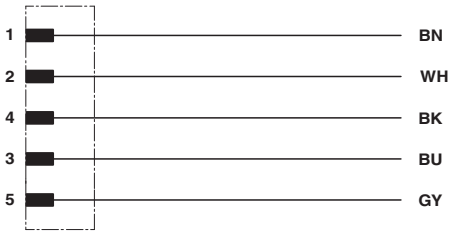
Contact assignment of the M12 plug
