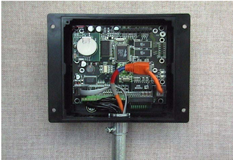
Figure B-10. Rear View of Intellicom with Outer Casing Showing Wiring from Conduit
