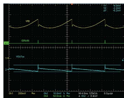
Figure 16. Output voltage ripple at 230 V IN_AC no load
