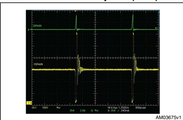
Figure 35. Operating with secondary winding shorted. Steady state (zoom)
