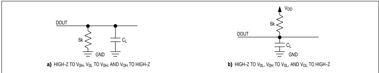
Figure 1. Load Circuits for Enable and Disable Time
