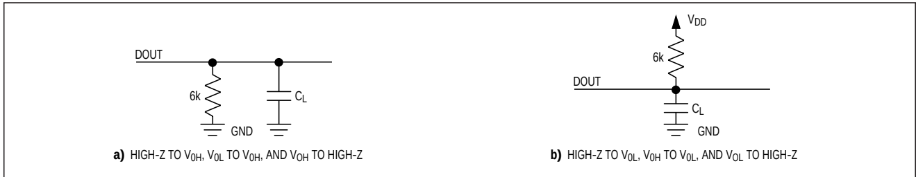
Figure 1. Load Circuits for Enable and Disable Time
