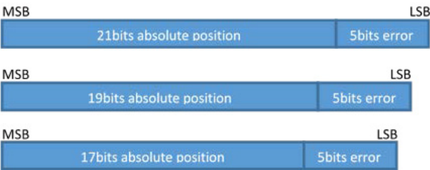
Figure 9: AR18 SSI 3-Wire Format Output
