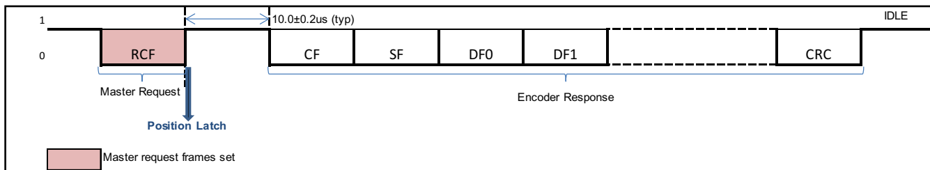
Figure 12: Encoder Data Read Out Frames Set
