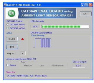
Figure 6. GUI - ADIM Mode, Device Enabled
