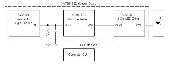
Figure 2. Ambient Light Sensor Mode Block Diagram
