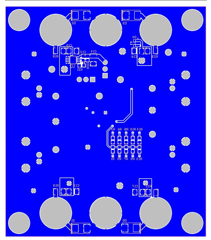
Figure 7. Bottom Layer (Power and Ground)
