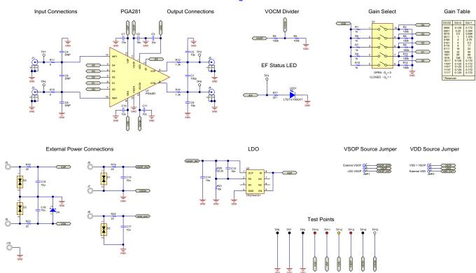
Figure 2. PGA281EVM Schematic
