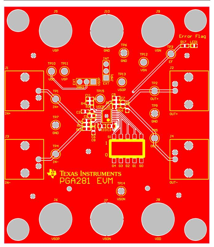
Figure 4. Top Layer (Signal and Ground)
