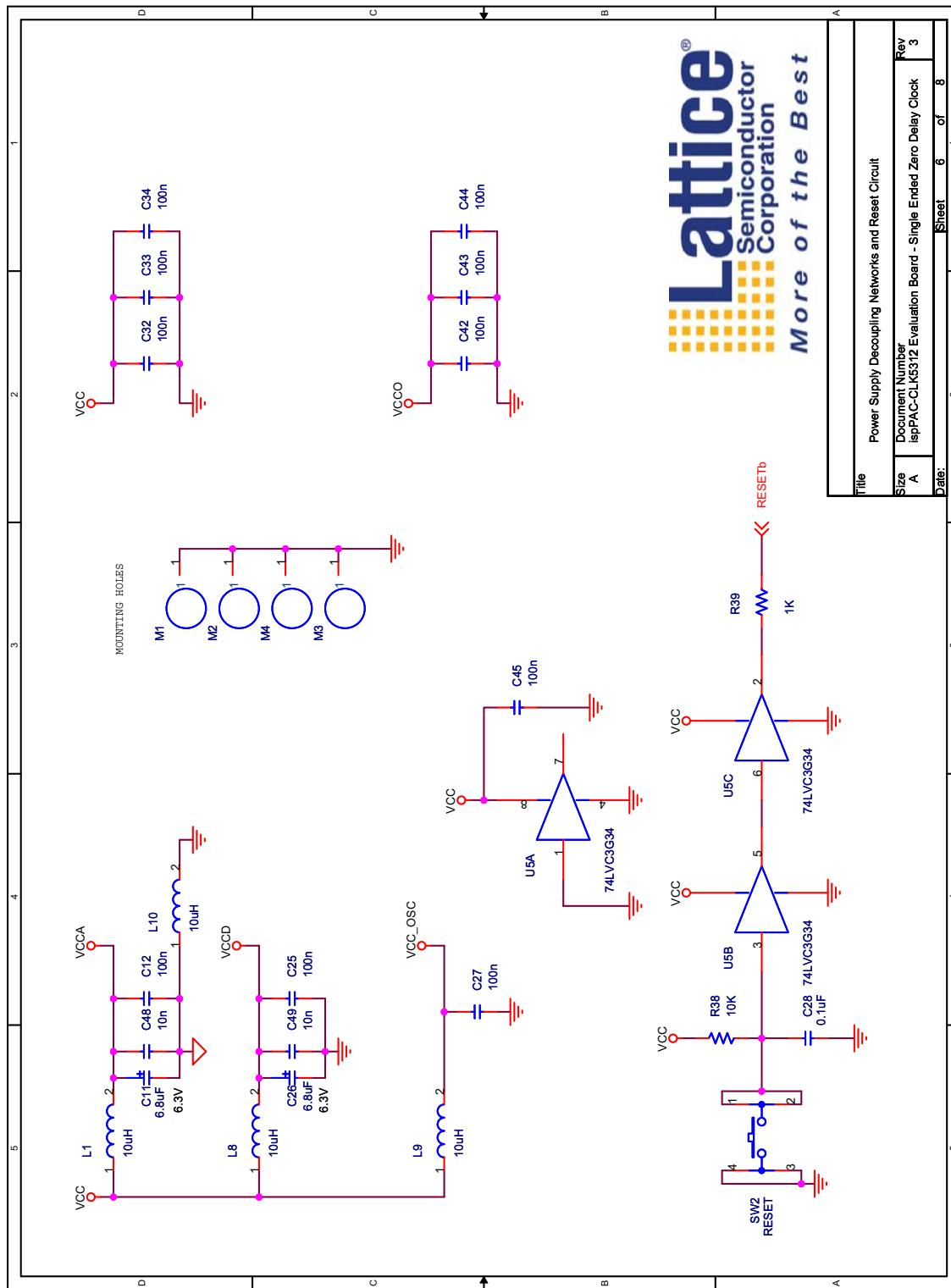
Figure 14. Banks 0, 1 and 2 Power Supply Decoupling Networks
