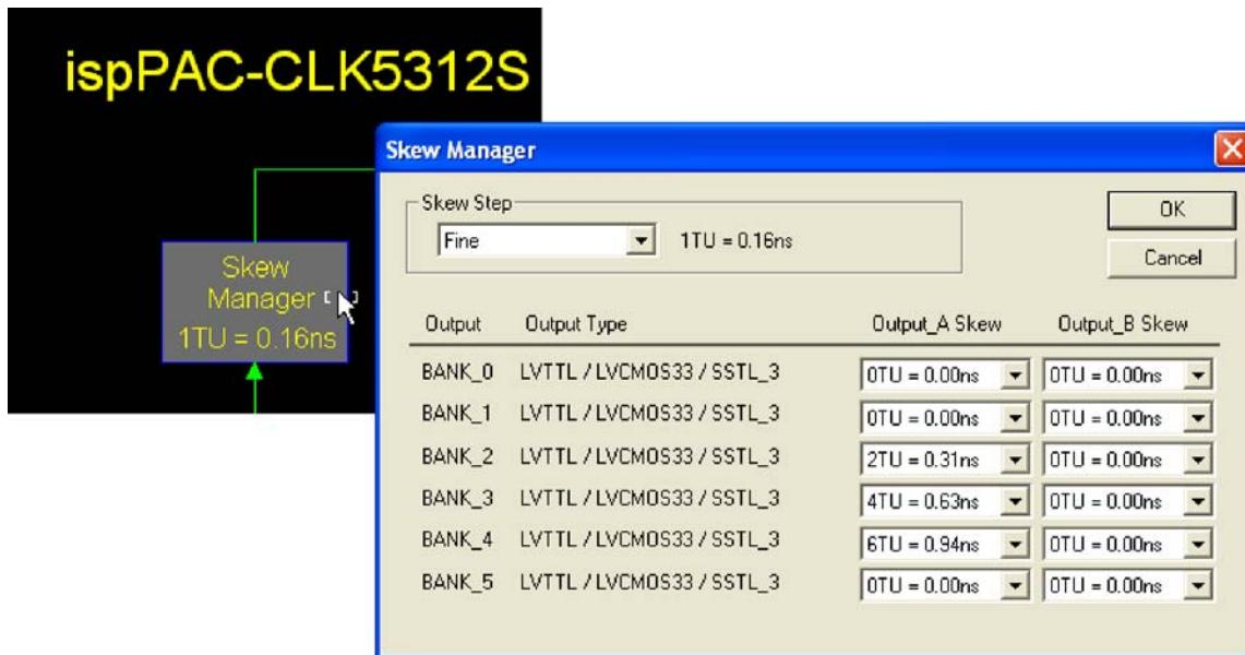
**Figure 7. Outputs are Skewed 300ps**
