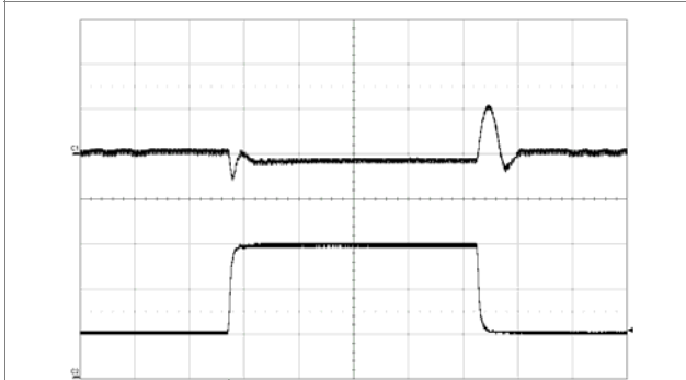
Output Load Transient Response, Default PID/NLR
