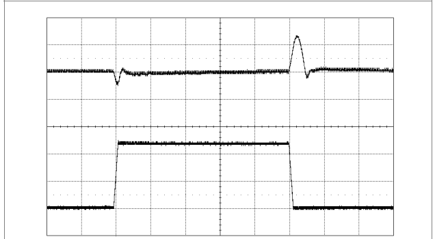
Output voltage response to load Step-change (12.5-37.5-12.5 A) at: T_{P1} = +25^\circ C , V_I = 12 V , V_O = 1.0 V di/dt = 2 A/\mu s , f_{sw} = 320 kHz C_O = 470 \mu F /10 m \Omega Top trace: output voltage (200 mV/div.). Bottom trace: load current (10 A/div.). Time scale: (0.1 ms/div.).
