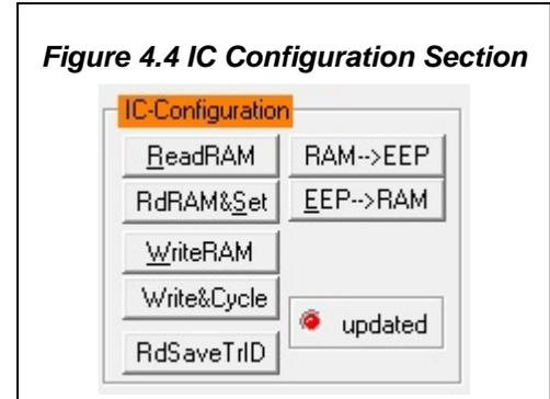
The “updated” virtual LED in the “IC Configuration” section displays the software configuration status compared to the attached ZSSC3154’s register content. If the content is identical, the LED is green (on).
