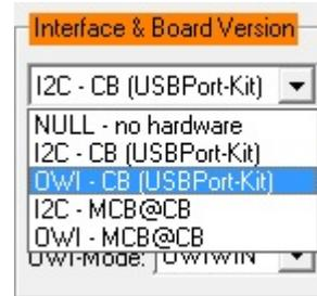
**Figure 4.3 Additional I<sup>2</sup>C™ and OWI Interface Settings in the “Send Command” Menu**
