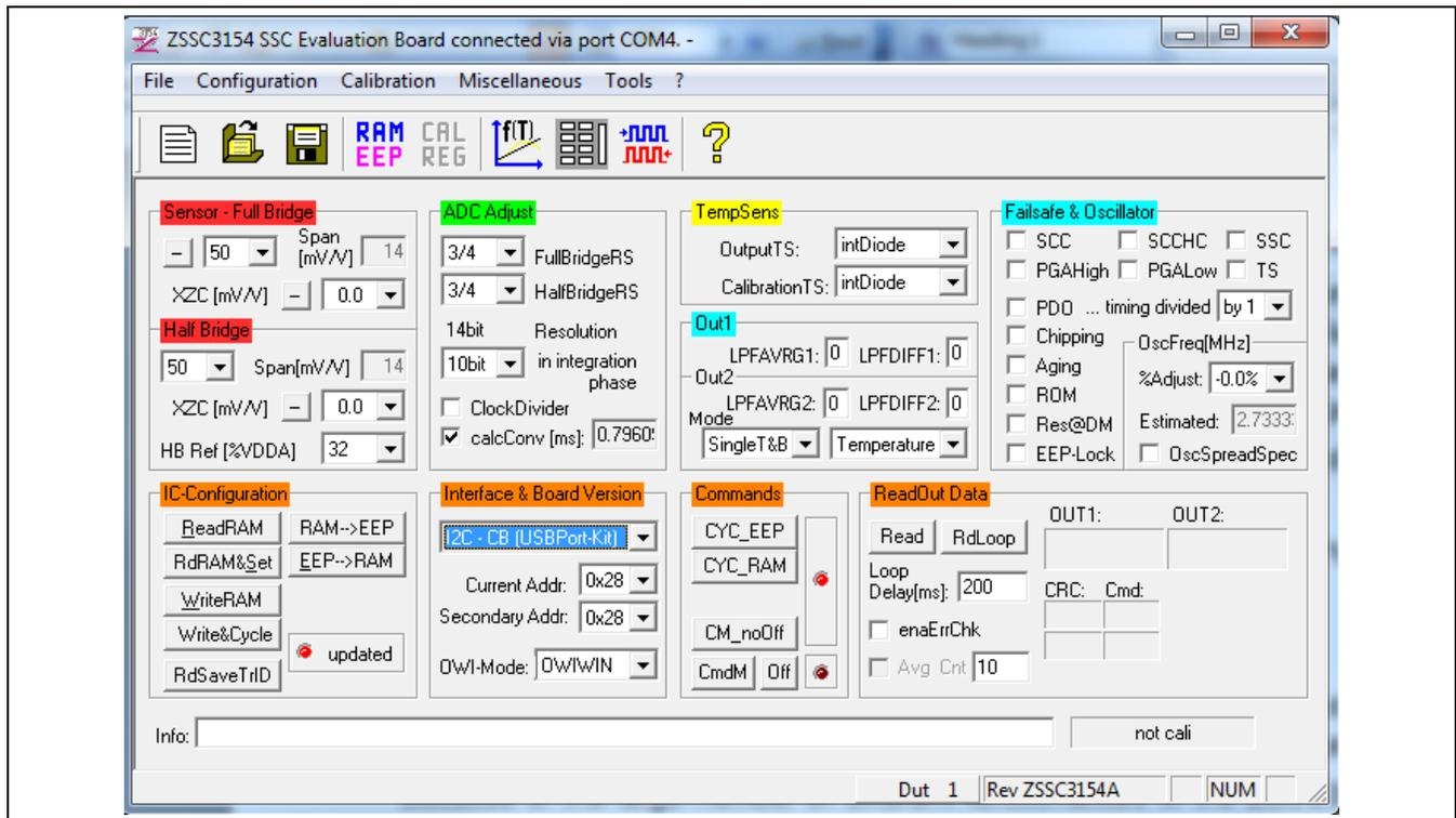
The main window includes all the settings for configuration of the ZSSC3154 in a clear structure that hides the corresponding HEX commands behind buttons and drop-down menus. For a detailed description of the commands, refer to the *ZSSC3154 Functional Description*. An information box that explains functionality appears when the cursor is placed over most buttons, drop-down menus, and check boxes.
