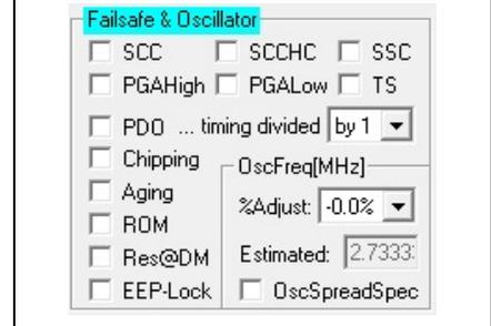
**SCC** : Enables Sensor Connection Check.
