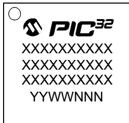
64-Lead QFN (9x9x0.9 mm)
