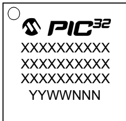
64-Lead QFN (9x9x0.9 mm)
