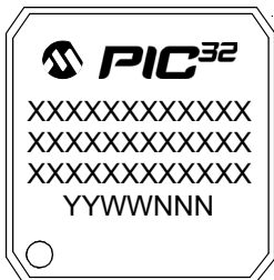
144-Lead TQFP (16x16x1 mm)
