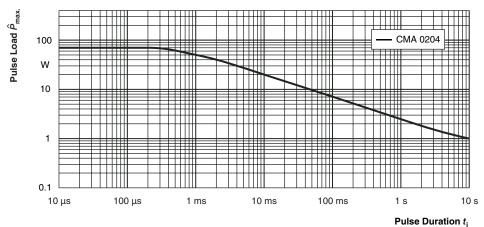
Maximum pulse load, single pulse; applicable if  $\overline{P} \rightarrow 0$  and  $n \le 1000$  and  $\hat{U} \le \hat{U}_{max}$ ; **Single Pulse** for permissible resistance change equivalent to 8000 h operation
