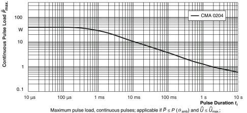
Maximum pulse load, continuous pulses; applicable if  $P \le P$  ( $\vartheta_{amb}$ ) and  $U \le U_{max}$ for permissible resistance change equivalent to 8000 h operation
