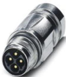
Coupler connector, straight, SPEEDCON locking, M17, Number of positions: 5+3+PE, Type of contact: Male connector, Crimp connection, shielded: yes, Cable diameter: 10 mm...12.5 mm
