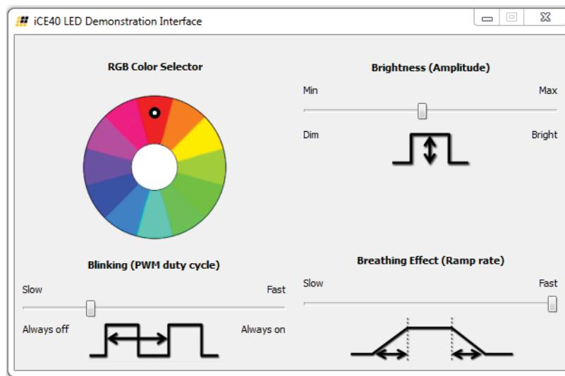
Now you can control the RGB LED on the iCE40 UltraLite Breakout Board. You can set the color, brightness, blinking rate as well as breathing.
