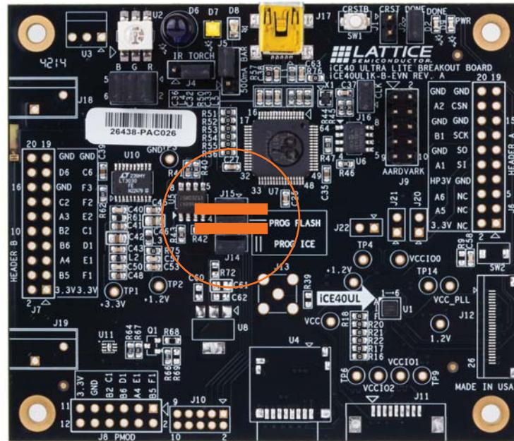
3. Connect the iCE40 UltraLite breakout board via the USB cable to a PC or MAC.
