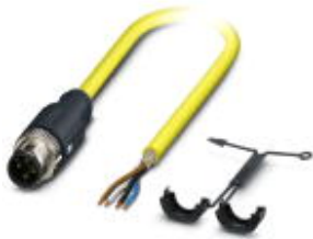
Sensor/Actuator cable, 4-position, PVC, yellow RAL 1021, shielded, Plug straight M12 SPEEDCON, A-coded, on free cable end, Cable length: 5 m
