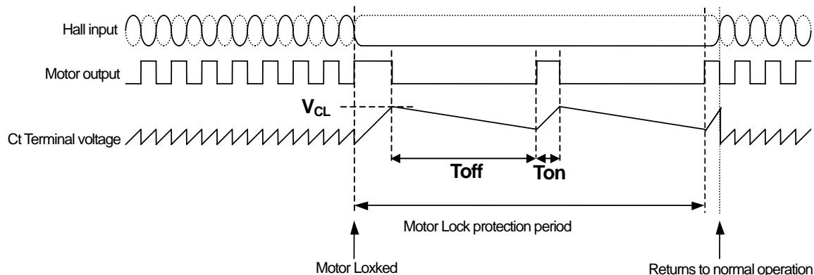
\*Remarks : When  $V_{DD}$  becomes lower than 4V, the Clamp Voltage( $V_{CL}$ ) becomes lower accordingly. This makes Ton and Toff shorter and may cause issues associated with the restarting of the motor from the lock protection state. Therefore, careful evaluation is necessary with actual motors.
