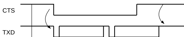
Figure 36-28. Transmitter Behavior when Operating with Hardware Handshaking
