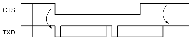
Figure 36-28. Transmitter Behavior when Operating with Hardware Handshaking
