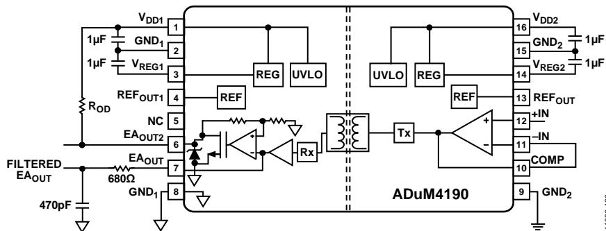
Figure 29. Test Circuit 3: Isolated Amplifier Circuit
