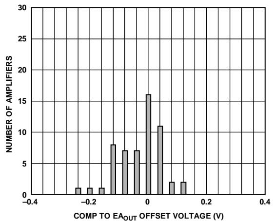
Figure 21. EA<sub>OUT</sub> Offset Voltage Distribution at -40°C
