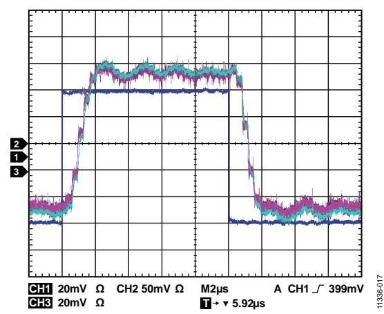
Figure 26. Output Square Wave Response with Test Circuit 3, Channel 1 = +IN, Channel 2 = EA<sub>out</sub>, Channel 3 = EA<sub>out2</sub>
