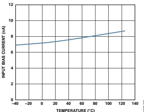
Figure 6.  $+IN, -IN$  Input Bias Current vs. Temperature
