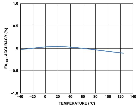
Figure 8.  $EA_{OUT}$  Accuracy vs. Temperature
