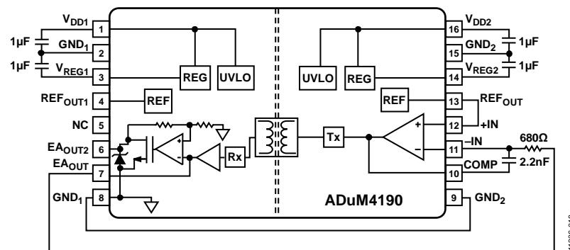
Figure 27. Test Circuit 1: Accuracy Circuit Using  $EA_{OUT}$
