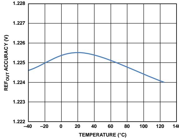
Figure 7.  $REF_{OUT}$  Accuracy vs. Temperature
