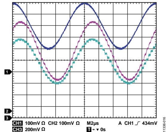
Figure 25. Output 100 kHz Signal with Test Circuit 3, Channel 1 = +IN, Channel 2 = EA<sub>out</sub>, Channel 3 = EA<sub>out2</sub>
