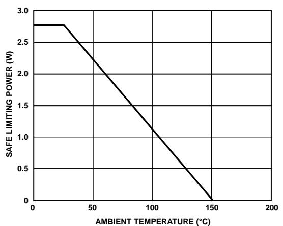
Figure 2. Thermal Derating Curve, Dependence of Safety Limiting Values on Case Temperature, per DIN V VDE V 0884-10
