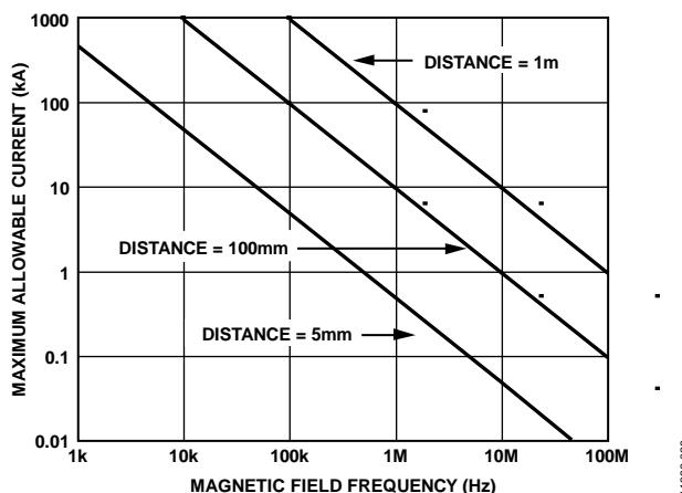
Figure 36. Maximum Allowable Current for Various Current-to-ADuM4190 Spacings
