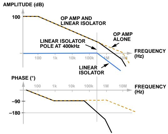
Figure 30. Bode Plot 1: Op Amp and Linear Isolator
