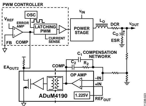
Figure 32. Application Block Diagram
