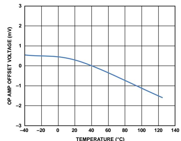
Figure 9. Op Amp Offset Voltage vs. Temperature
