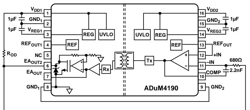
Figure 28. Test Circuit 2: Accuracy Circuit Using  $EA_{OUT2}$
