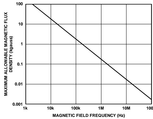
Figure 35. Maximum Allowable External Magnetic Flux Density
