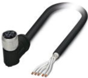
Sensor/Actuator cable, 5-position, PE-X halogen-free, black, shielded, free cable end, on Socket angled M12 SPEEDCON, A-coded, Cable length: 2 m, For railway applications
