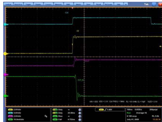
Figure 17: Turn OFF output current characteristics (2)
