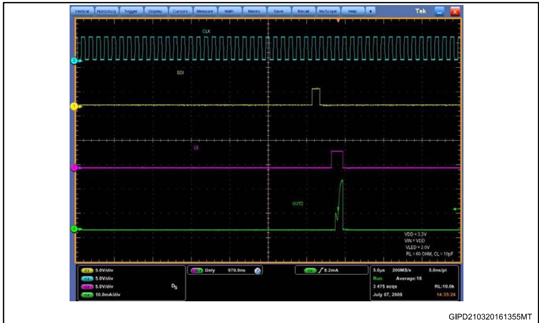
Figure 19: First output ON after switching from auto power saving to normal operating condition
