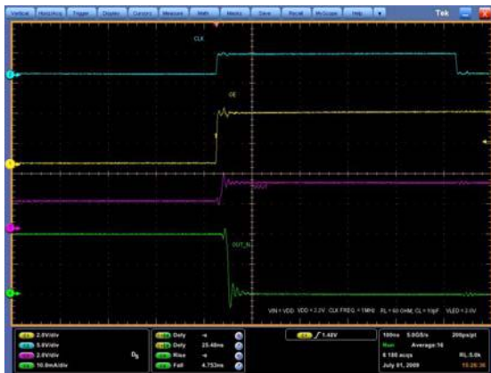
Figure 16: Turn ON output current characteristics (1)
