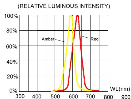
FIG.4 RELATIVE LUMINOUS INTENSITY VS.
