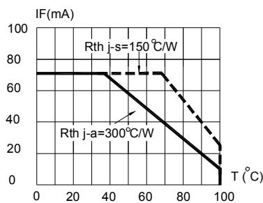
FIG.5 RED&AMBER MAXIMUM FORWARD DC CURRENT VS AMBIENT
