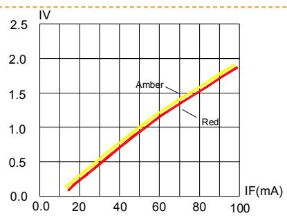
FIG.2 RELATIVE LUMINOUS INTENSITY VS.
