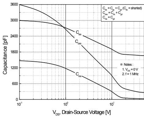
**Figure 5. Capacitance Characteristics**
