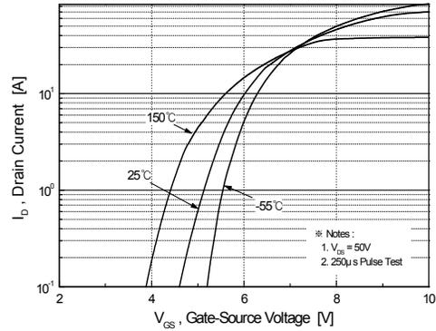
**Figure 2. Transfer Characteristics**
