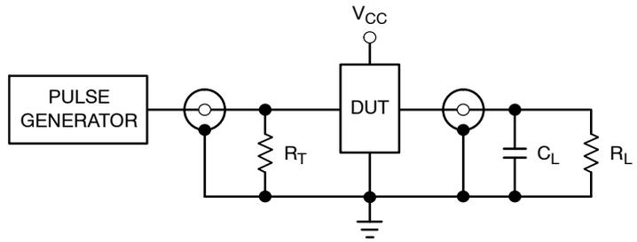
$R_T = C_L$  or equivalent (includes jog and probe capacitance)
