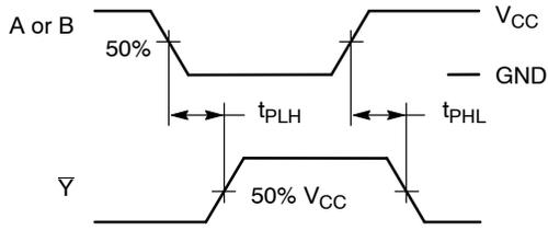
Figure 3. Switching Waveforms
