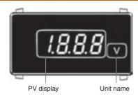
Select the decimal position with terminal 12, 13, or 14 on the rear panel.
