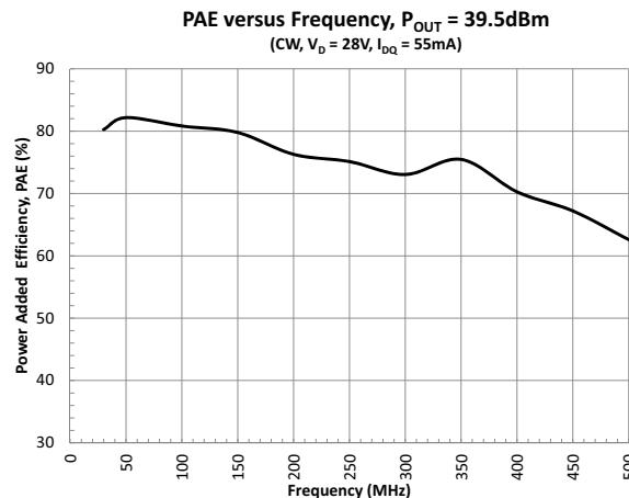
**Typical Performance in standard fixed tuned test fixture matched for 30MHz to 512MHz (T = 25 °C, unless noted)**
