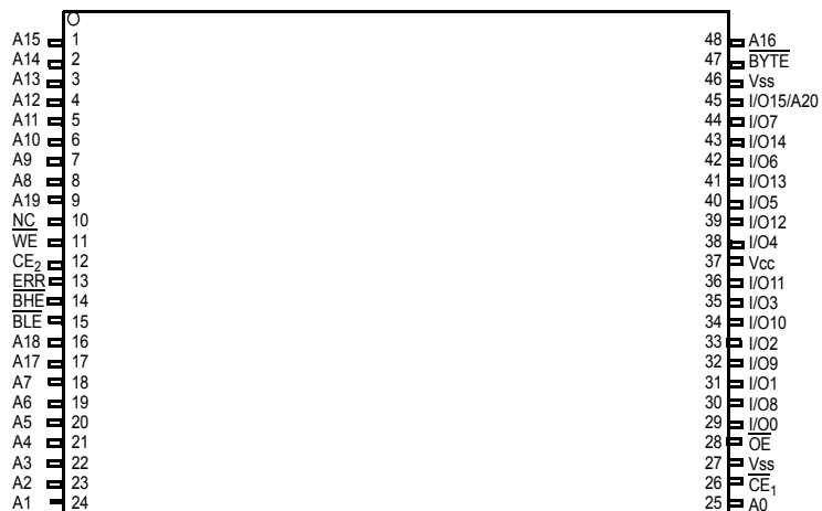
Figure 5. 48-pin TSOP I Pinout (Dual Chip Enable with ERR) – CY62167GE [7, 8]
