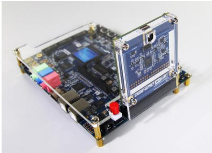
Figure 1-4 Connect the D8M to C5G board's expansion port
