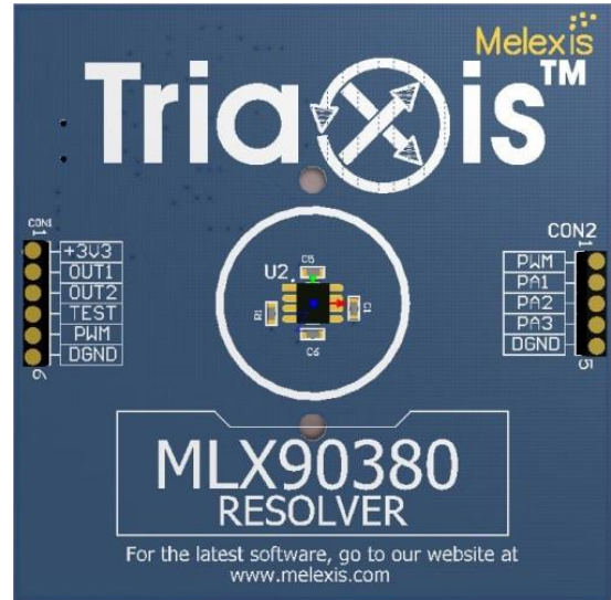
Figure 1: MLX90380 Resolver Evaluation/Demonstration board
