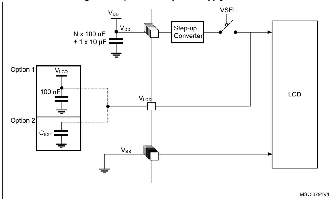
1. Option 1: LCD power supply is provided by a dedicated  $V_{LCD}$  supply source,  $V_{SEL}$  switch is open.
