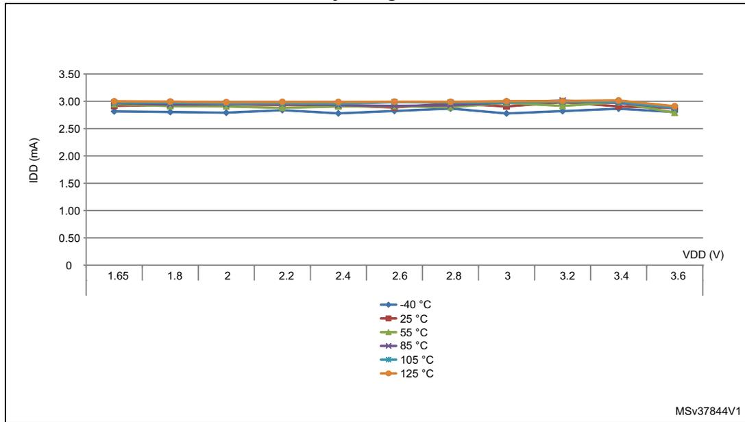
Table 32. Current consumption in Run mode, code with data processing running from RAM
