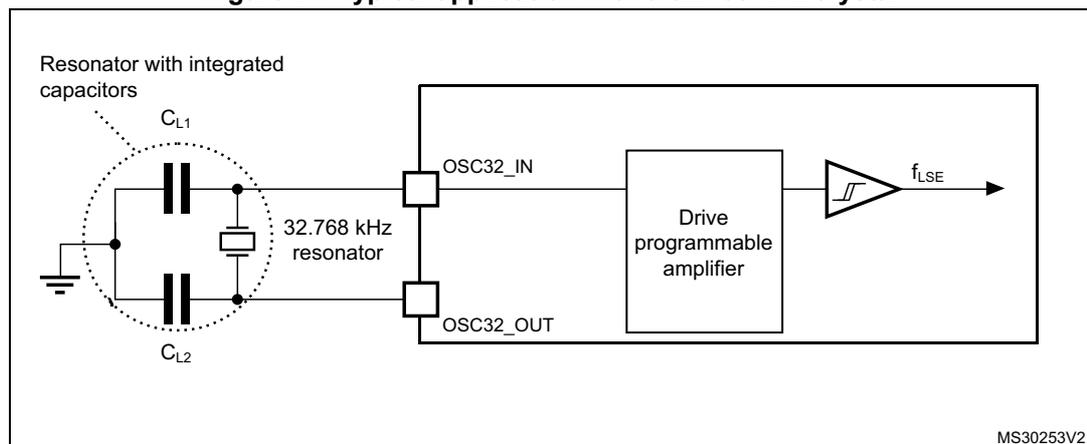
**Note:** An external resistor is not required between  $OSC32\_IN$  and  $OSC32\_OUT$  and it is forbidden to add one.
