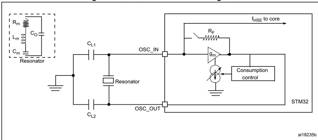
**Low-speed external clock generated from a crystal/ceramic resonator**
