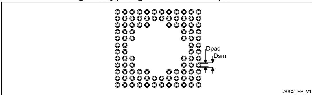
**Table 84. UFBGA100 recommended PCB design rules (0.5 mm pitch BGA)**
