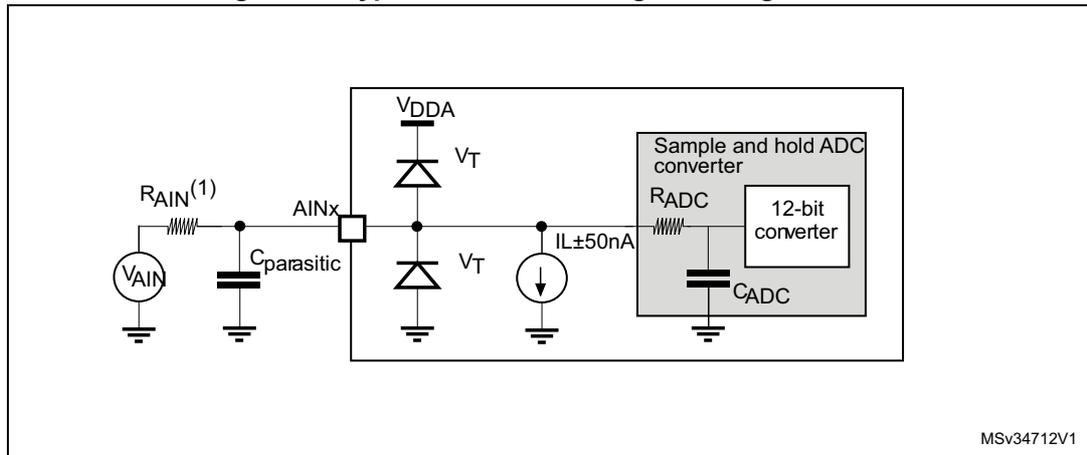
1. Refer to [Table 64: ADC characteristics](#) for the values of  $R_{AIN}$ ,  $R_{ADC}$  and  $C_{ADC}$ .
