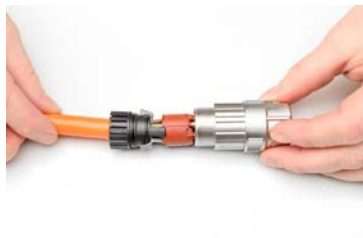
Step 15 - Push sub-assembly into shell
