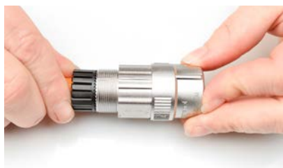
Step 15 - Push sub-assembly into shell
