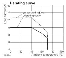
Other standards: the test conditions (e.g. UL508) differ from the EN standard, hence under these conditions other temperature/current combinations may be permissible; please contact our technical support for details. In case no derating curves are given, the indicated temperature and load current refer to the approved standards for the specific product and not to the EN61984.
