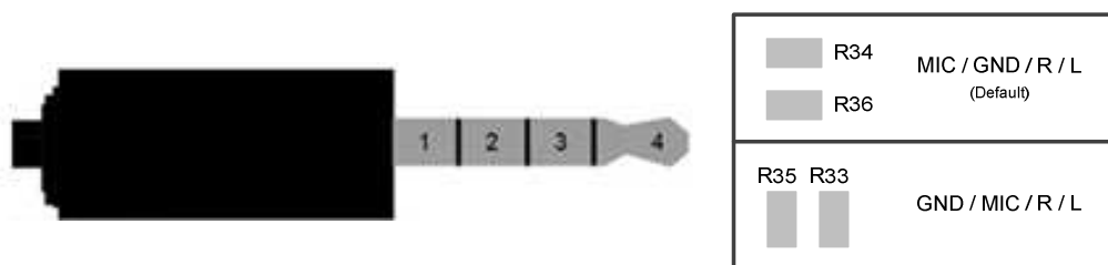
Figure 2 Headset Jack Configuration Options
