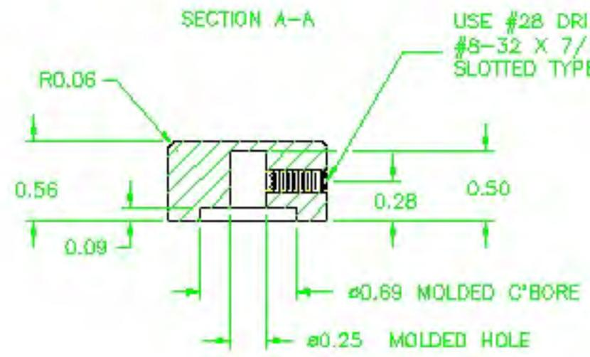
USE #28 DRILL (0.140), #8-32 TAP, #8-32 X 7/16 LG. CUP POINTED, SLOTTED TYPE, SET SCREW 10022.
