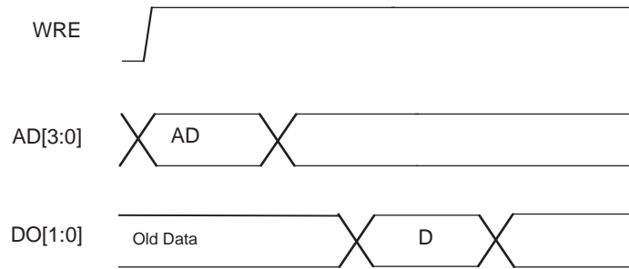
Figure 3-7. Slice Single /Dual Port Read Cycle Timing
